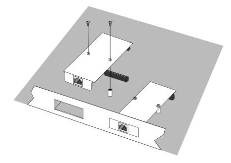
Figure 2-1. Installing an FPIM
